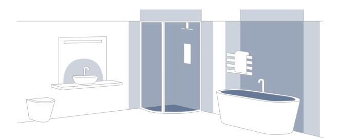
When installing Waves in the bathroom, you have to take into account that the bathroom is divided into 4 zones (0-3). Based on the IP class, the device can be placed in zones 2 or 3.
